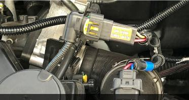
Step 4: The tuning box connectors are applied to the Boost sensor
