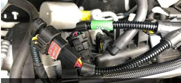
Step 3: The tuning box connectors are applied to the MAP sensor
