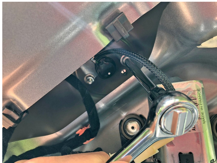
Step 4: Remove both 10mm nuts to release the mechanism
