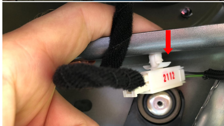
Step 2: Pop-out the wiring connector with your finger
