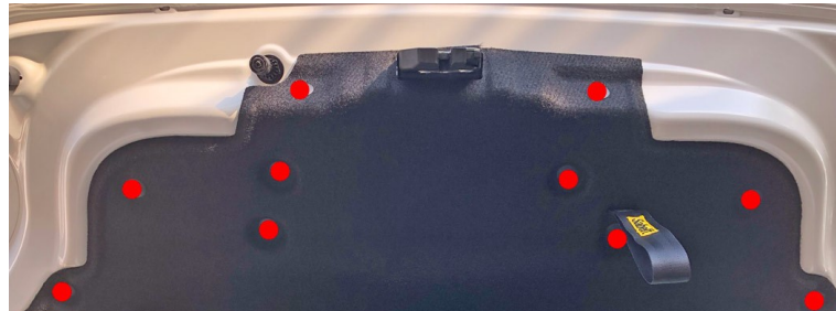
Step 1: Remove tailgate trim by gently easing off the ten clips
