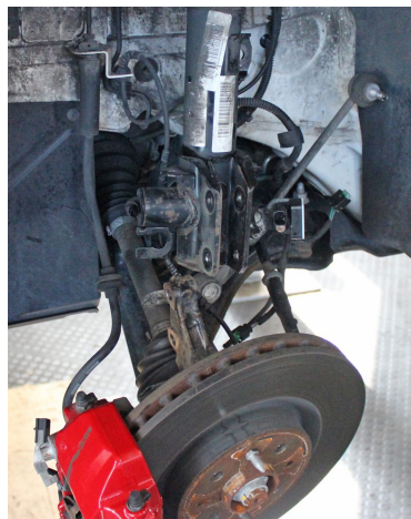
Pic. 2.3. Undo the top of the drop link and move to the side
