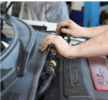
Pic. 1.2. Rubber pieces both sides and remove wiring clip
