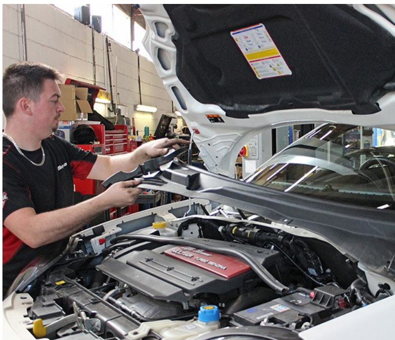
Pic. 3.2a. Carefully re-position the scuttle ready for fitting
