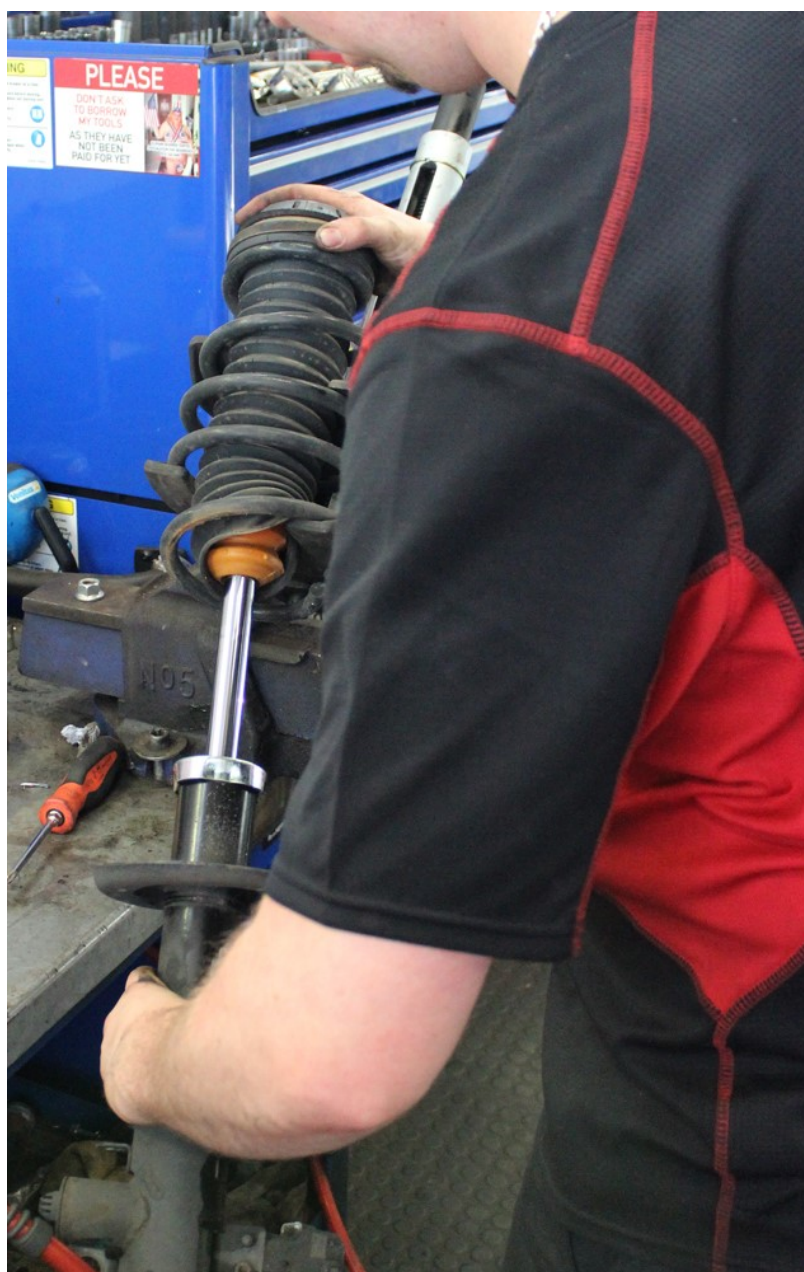
Pic. 2.8. With the top nut undone and the constituent parts removed, simply remove the shock absorber from below
