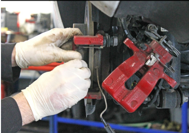
Pic. 6. Remove anti-rattle springs
