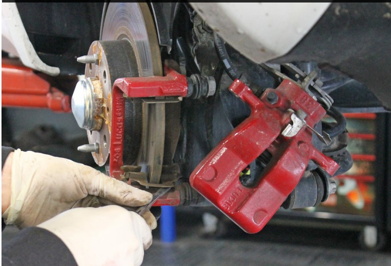
Pic. 9. Winding back the piston with the wind-back tool
