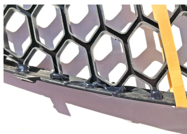
Pic. 8.1. Use elastic bands to hold the grille together before gluing
