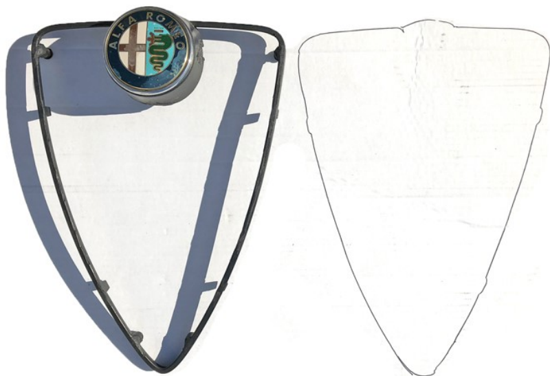
Pic. 5.1. Carefully draw round the outside grille onto cardboard
