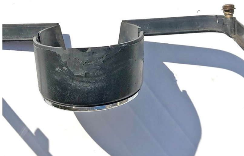
Pic. 4.2. Take care to achieve a flat surface, but gently round off the plastic around the four screws - do not take off too much plastic!
