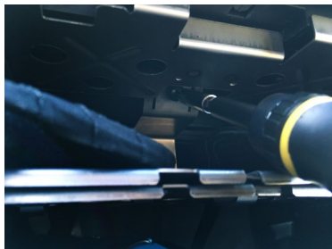
Step 3: ISO keys also used to remove Blue&Me unit
