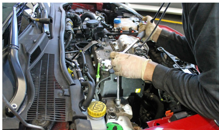
Pic. 4.5(a) Remove three 18mm side engine mount bolts
