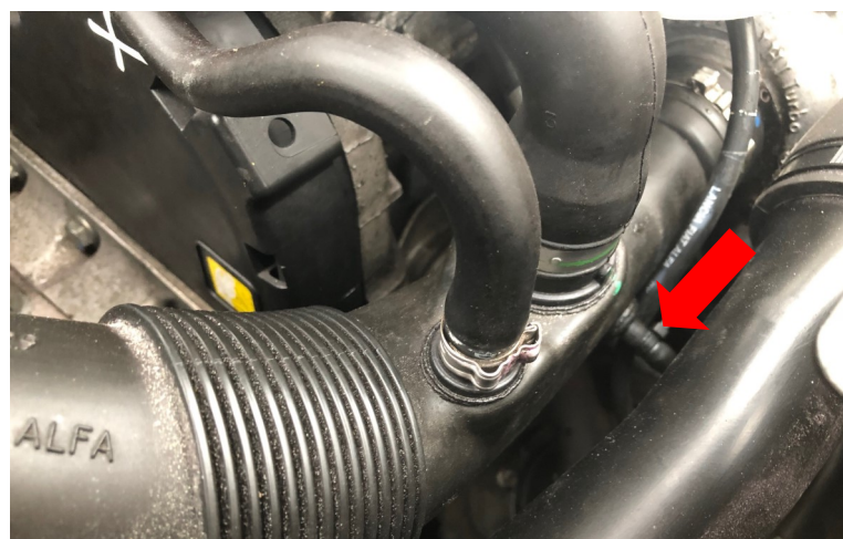
Pic. 2.5(b) This hose has a sacrificial/single use clamp and needs to be replaced with a cable tie when re-fitting
