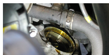
Pic. 2.6 Remove oil filter housing with 27mm socket
