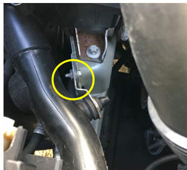
Pic. 2.5(a) Remove breather rail, air pipework and airbox
