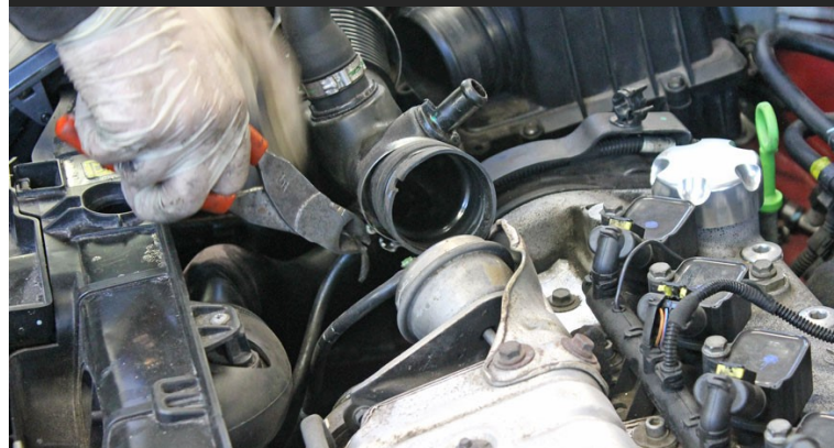
Pic. 6.9 Refit air pipework and hoses, ensuring the lower hose shown below is held with a new cable tie
