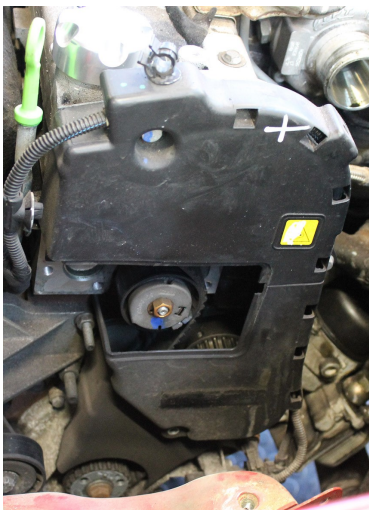
Pic. 4.5(b) Remove three 15mm engine mount bolts
