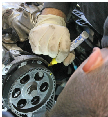
Pic. 4.6 Finally the cambelt, cambelt tensioner and water pump are visible with the plastic cambelt covers removed
