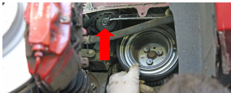
Pic. 4.2 Holding the auxiliary belt tensioner with a 13mm spanner, push and hold down clockwise to release tension on the belt
