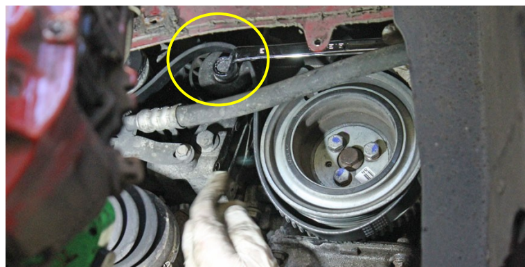
Pic. 6.7 Fit new auxiliary belt by slackening off the tensioner
