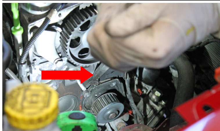
Pic. 5.1(b) Prise the water pump away from the engine casing
