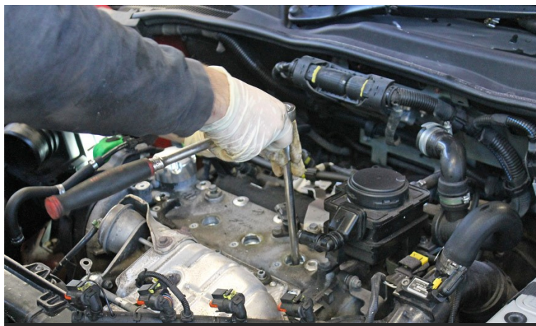
Pic. 3.4 Remove all four spark plugs with 16mm plug socket
