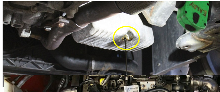
Pic. 2.4 - Oil drain plug at the rear of the engine sump
