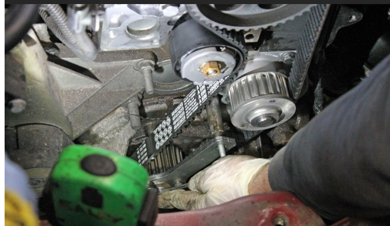
Pic. 6.3 Unbolt the crankshaft locking tool
