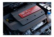
features a little-known (and quite well hidden) MultiAir filter which is separate from the usual oil filter. Many owners, garages and even some dealers do not understand the importance of this which contributes to MultiAir unit failures (approximately £500 to replace, plus labour). Symptoms are misfires and roughrunning, so only buy a MiTo with a comprehensive service history
