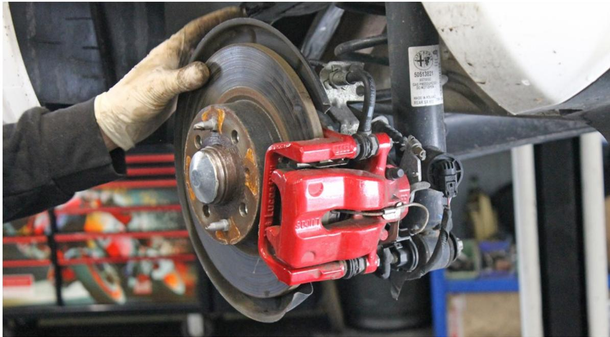
Brembo calipers which use 305mm discs.
