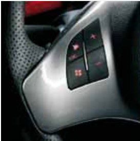
Remote audio controls on steering wheel
