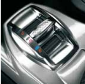
Alfa Romeo D.N.A. (vehicle's dynamic control switch)
